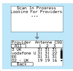
For a reliable 2/3/4G connection it is recommended that for the chosen network (SIM card) used there should be at least two base stations with signal strength (CSQ) of 10 or more.
